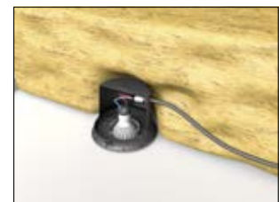
4. Insulation material can now be applied.
